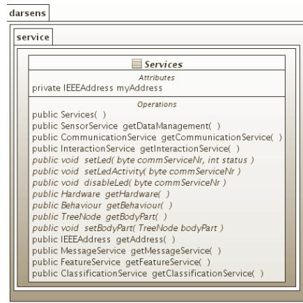
Figure 4.3: UML diagram of the Service class
